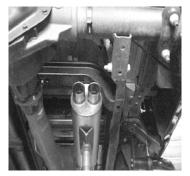
CONNECT MUFFLER WITH THE INLET TOWARDS THE CONVERTER. MAKE SURE REAR OF MUFFLER OUTLETS SIT AT 3 AND 9 O'CLOCK. ALLOW A MINIMUM OF 1 ½" TO SLIDE OVER THE HEADPIPE. USE A JACKSTAND TO SUPPORT THE MUFFLER AND CONNECT CLAMP # G. DO NOT TIGHTEN.
