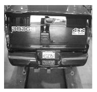
WHEN YOU HAVE EVERYTHING IN PLACE. MAKE SURE YOU HAVE A 1" CLEARANCE ON ALL PIPES ETC. FIRMLY TIGHTEN ALL BOLTS AND CLAMPS. USE ZIP TIES TO SECURE BACK VENT LINES AND BRAKE LINES. INSTALL STAINLESS TIPS.
