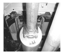
INSTALL MUFFLER ONTO STOCK HEADPIPE AND ATTACH WITH FRONT MUFFLER HANGER # I AND INSERT INTO RUBBER GROMMETS. ALIGN NOTCH ON GIBSON MUFFLER TO STOCK ALIGNMENT PIN ON FACTORY HEADPIPE. MUFFLER INLET IS TOWARDS THE CONVERTER .USE A JACK STAND TO SUPPORT THE MUFFLER.
