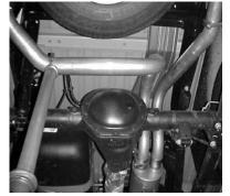
INSTALL PASSENGER SIDE OVERAXLE PIPE #D AND ATTACH TO MUFFLER USING CLAMP # F. ATTACH HANGER # H AND CLAMP #F TO OVERAXLE TAILPIPE.
