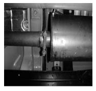
DO NOT REMOVE THE FACTORY EXTENSION PIPE BETWEEN THE MUFFLER AND THE CONVERTER. REMOVE THE FIRST CLAMP IN FRONT OF YOUR STOCK MUFFLER. UNBOLT AND REMOVE STOCK REAR HANGER ON PASSENGER SIDE FRAME RAIL. THEN REMOVE STOCK EXHAUST. USE WD-40 ON ALL HANGERS AND LEAVE ALL RUBBER GROMMETS IN PLACE.
