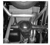
INSTALL OVERAXLE PASSENGER TAILPIPE #E TO OUTLET OF MUFFLER WITH CLAMP #I. SPARE TIRE MAY NEED TO BE LOOSENED AND PUSHED TO THE REAR OF THE TRUCK FOR CLEARANCE PURPOSES... INSTALL DRIVER SIDE OVERAXLE TAILPIPE #C AND #D, AND CLAMP DOWN HANGER #H TO MUFFLER & TAILPIPE. USE CLAMP #I TO CONNECT BOTH PIPES. DO NOT TIGHTEN!
