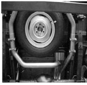
USE ZIP TIES TO TIE BRAKE LINES, WIRES, ETC. AWAY FROM ALL PIPES. KEEP IN MIND THAT YOU WILL NEED TO ROTATE PIPES TO BEST FIT YOUR TRUCK. AFTER YOU HAVE EVERYTHING POSITIONED. TIGHTEN ALL CLAMPS. INSTALL STAINLESS TIPS.
