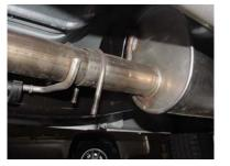
TO REMOVE STOCK EXHAUST UNCLAMP IT FROM THE CLAMP LOCATED JUST IN FRONT OF YOUR STOCK MUFFLER, YOU MAY NEED TO HEAT IT UP WITH A TORCH TO REMOVE IT. NOW CUT OFF YOUR STOCK TAILPIPE JUST BEHIND THE MUFFLER AND REMOVE.LEAVE ALL RUBBER GROMMETS ON THE HANGER. USE WD-40 TO AID IN REMOVAL OF EXHAUST AND HANGERS.
