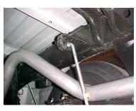
INSTALL PASSENGER SIDE TAILPIPE #C INTO MUFFLER 1-1/2" TO 2". USE CLAMP #G TO SECURE TAILPIPE TO MUFFLER. INSERT WELDED HANGER INTO RUBBER GROMMET. DO NOT TIGHTEN
