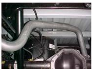
SPARE TIRE MAY NEED TO BE LOOSENED AND PUSHED TO THE REAR OF THE TRUCK FOR BETTER CLEARANCE.
