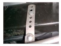
MEASURE 19 ½" FROM THE REAR OF THE FRAME AND USE THIS HOLE AND BOLT ON HANGER #F. USE THE 3<sup>RD</sup> HOLE FROM THE TOP.
