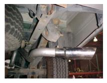
INSTALL DRIVERSIDE FRONT TAILPIPE #B INTO MUFFLER AT LEAST 1 1/2" TO 2".USING CLAMP # F. NEXT INSTALL DRIVERSIDE OVERAXLE PIPE # C TO FRONT TAILPIPE USING CLAMP # F DO NOT TIGHTEN
