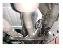
INSTALL HEADPIPE #A, YOU WILL NEED TO LINE UP THE TWO NOTCHES. INSERT WELDED HANGER INTO RUBBER GROMMET. USE CLAMP #H TO SECURE HEADPIPE TO THE STOCK PIPE. DO NOT TIGHTEN.
