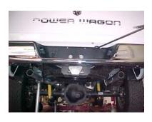
MEASURE 19 ½" FROM THE REAR OF THE FRAME AND USE THIS HOLE AND BOLT ON HANGER #F. USE THE 1<sup>ST</sup>. HOLE FROM THE TOP. IT WILL BOLT ON THE INSIDE OF THE FRAME.
