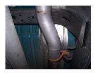
3. Install headpipe #A onto your existing stock headpipe and secure with clamp #G. Use a jack stand to support the converter.
