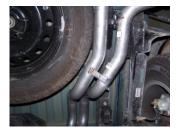
8. Attach tailpipes together with bolt kit #I. Do not tighten. Driver side tabs will be on the bottom.
