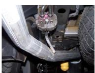
**6.** Remove spare tire to install tailpipes (Reference vehicle manual for removal of spare tire). Now install Driver side tailpipe #D into the muffler 1½-2". Use clamp #H to secure tailpipe to muffler. DO NOT TIGHTEN. Insert welded hangers into rubber grommets.
