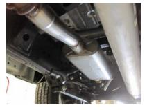
1. Disconnect the negative battery cable before removal of OEM exhaust. This will allow the computer to reset and recognize the new exhaust. Lay out the exhaust on the floor so it looks like the drawing and compare parts with manual.
