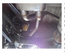
**4.** Install muffler #B onto head pipe #A  $1\frac{1}{2}$ "-2". Use a jack stand to support the muffler. Use clamp #G to secure the muffler to the headpipe. DO NOT TIGHTEN.
