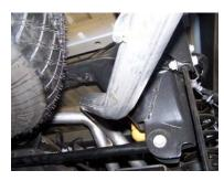
**7.** Install Passenger side tailpipe #C into the muffler 1½-2". Use clamp #H to secure tailpipe to muffler. DO NOT TIGHTEN. Insert welded hangers into rubber grommets.
