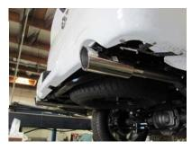
**9.** Install stainless steel tips #F. Clamp down. When you have everything in place and clear from all brake lines, shocks, etc. firmly tighten all bolts and clamps down securely beginning from the front. Inspect all fasteners after 25-50 miles of operation and re-tighten as necessary.
