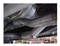
Install head pipe #A onto passenger side stock pipe and insert hanger into rubber grommet. Next install driver side head pipe #B onto drivers side factory pipe. Use clamp #H to secure pipes to factory pipes. Do not tighten.
