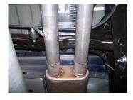
5. Install extension pipe #D into muffler. Use clamp #I to secure. Do not tighten. Next install driver side extension pipe #E into muffler using clamp #I to secure. Do not tighten. Insert welded hanger into rubber grommet.
