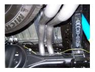
7. Install driver side overaxle tailpipe #G onto extension pipe. Use clamp #I to secure the pipe. Do not tighten.
