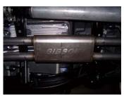
4. Install muffler onto headpipes 1.5"-2" with the louvers facing towards the converter. Use a jack stand to support the muffler. Use clamps #I to secure the muffler to the headpipes. Do not tighten. Muffler inlet is looking into the louvers.
