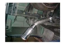
INSTALL EXIT PIPES # E ONTO TAILPIPES USE CLAMP # I TO SECURE PIPES TOGETHER CLAMP ON, DRIVERS SIDE WILL HOOK UP TO THE REAR HANGER TO HOLD PIPES UP.
