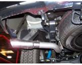
7. Install rear tailpipe hanger #K. Use bolt kit #L to secure. Use the hole on frame closest to the rear shackle. Install rubber grommet on rear hanger.
