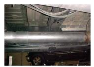
NEXT, INSTALL RESONATOR # B 1 1/2"-2" ONTO Y-PIPE USE CLAMP # I TO SECURE PIPES TOGETHER, DO NOT TIGHTEN.
