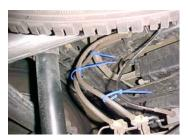
MAKE SURE YOU HAVE A 1" CLEARANCE ON ALL RUBBER BRAKE LINES, SHOCK BOOTS, TIRES, FUEL LINES, ETC...
