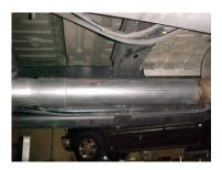
NEXT, INSTALL RESONATOR # B 1 ½"-2" ONTO Y-PIPE USE CLAMP # G TO SECURE PIPES TOGETHER, DO NOT TIGHTEN.
