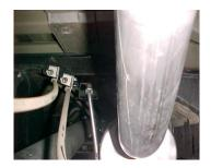
INSTALL BAND CLAMP # I ONTO MUFFLER, INSERT HANGER INTO RUBBER GROMMET, USE BOLT KIT PROVIDED, DO NOT TIGHTEN.
