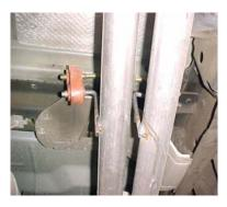
INSTALL THE DRIVERSIDE FRONT TAILPIPE # D TO OUTLET OF MUFFLER 1.5" TO 2". THE TAILPIPE INLET THAT GOES INTO THE MUFFLER IS 4.5" LONG. INSERT HANGER INTO RUBBER GROMMET. ATTACH WITH HANGER# G. INSTALL DRIVERSIDE OVERAXLE TAILPIPE # E TO FRONT DRIVERSIDE TAILPIPE, THIS PART HAS A SWEDGE UP ON IT. ATTACH USING CLAMP # G.
