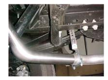
INSTALL PASSENGER SIDE OVERAXLE PIPE #C INTO MUFLER 1 ½" TO 2". USE CLAMP # I TO SECURE. DO NOT TIGHTEN. ROTATE UNTIL PIPE TOUCHES HANGER. USE CLAMP #I TO HOLD PIPE TO HANGER. DO NOT TIGHTEN.
