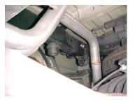
INSTALL PASSENGER SIDE TAILPIPE # C INTO MUFFLER 1 <sup>1</sup>/<sub>2</sub>" TO 2". INSERT WELDED HANGER INTO RUBBER GROMMET. USE CLAMP # H TO SECURE PIPE TO MUFFLER, DO NOT TIGHTEN. ROTATE PIPE TOWARDS DRIVERSIDE.
