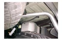
INSTALL DRIVERS SIDE TAILPIPE # D INTO MUFFLER 1½" TO 2". INSERT WELDED HANGERS INTO RUBBER GROMMETS. USE CLAMP # H TO SECURE PIPE TO MUFFLER, DO NOT TIGHTEN.
