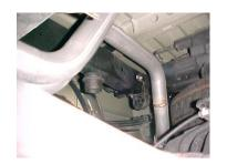
INSTALL PASSENGER SIDE TAILPIPE # C INTO MUFFLER  $1\frac{1}{2}$ " TO 2". INSERT WELDED HANGER INTO RUBBER GROMMET, USE CLAMP # H TO SECURE PIPE TO MUFFLER. DO NOT TIGHTEN. ROTATE PIPE TOWARDS DRIVERSIDE.
