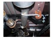
INSTALL HEADPIPE #A INTO STOCK PIPE. THE END OF THE PIPE SHOULD BE AT THE 12 O'CLOCK POSITION, ATTACH WITH FACTORY CLAMP. DO NOT TIGHTEN. INSERT WELDED HANGER INTO RUBBER GROMMET.
