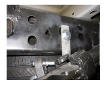
ON DRIVER SIDE: ATTACH REAR TAILPIPE HANFGER #I TO FRAME USING BOLT KIT PROVIDED
