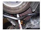
**6.** Install the driverside overaxle tailpipe #D into the muffler 1½-2". Use clamp #H to secure. DO NOT TIGHTEN. Rotate until it meets with the rubber grommet, use clamp #H to hold pipe. DO NOT TIGHTEN.
