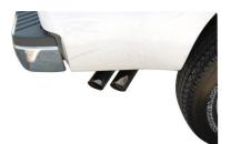
INSTALL YOUR STAINLESS TIPS. TIGHTEN ALL CLAMPS STARTING FROM THE FRONT, WORKING YOUR WAY TO THE BACK OF THE TRUCK. TO CLEAN TIPS USE A STAINLESS STEEL CLEANER & SCOTCH BTIE PAD.
