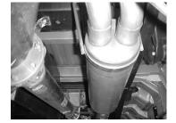
SLIP MUFFLER #B ONTO THE HEADPIPE 1 ½" TO 2". THE OUTLETS WILL BE LEVEL. USE CLAMP #G TO SECURE MUFFLER TO HEADPIPE. DO NOT TIGHTEN.
