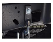
**5.** Install hanger #I into hole that is already threaded to receive the bolt Item# J on the driverside frame rail just rear of the axle. You will use the lower right side bolt hole. There will be 4 choices in the correct area. DO NOT TIGHTEN. Install rubber grommet
