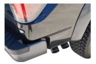
Install stainless steel tips. Clamp down. When you have everything in place, firmly tighten all bolts and clamps down securely. Use stainless steel cleaner and a Scotch Brite pad weekly to prevent tip from discoloration.
