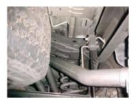
Install passenger side tailpipe # D into muffler 1-1/2" to 2", use clamp # I to secure. Do not tighten. Slide welded hanger into rubber grommet.
