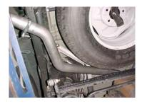
Next, install drivers side tailpipe # C into muffler 1-1/2" to 2" route between spare tire and shocks use clamp # G to secure, do not tighten.
