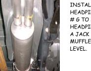
INSTALL MUFFLER # B ONTO HEADPIPE 1  $\frac{1}{2}$ " TO 2". USE CLAMP # G TO SECURE MUFFLER TO HEADPIPE. DO NOT TIGHTEN. USE A JACK STAND TO HOLD UP THE MUFFLER. OUTLETS SHOULD BE LEVEL.
