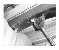
INSTALL WELDED HANGER INTO RUBBER GROMMET
