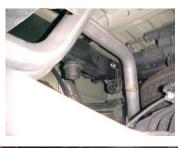
INSTALL PASSENGER SIDE TAILPIPE # C INTO MUFFLER 1 ½" TO 2". INSERT WELDED HANGER INTO RUBBER GROMMET, USE CLAMP # H TO SECURE PIPE TO MUFFLER. DO NOT TIGHTEN. ROTATE PIPE TOWARDS DRIVERSIDE.
