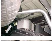
INSTALL DRIVERS SIDE TAILPIPE # D INTO MUFFLER 1 ½" TO 2". INSERT WELDED HANGERS INTO RUBBER GROMMETS. USE CLAMP # H TO SECURE PIPE TO MUFFLER, DO NOT TIGHTEN.
