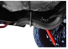
8. To install your XT Tip simply remove the exhaust from the Gibson head pipe and re install the tip using the same clamp and driver side only hanger. Protect your tips when in storage. We do not want any dings or dents.
