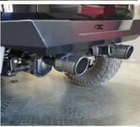
7. Adjust the tips to your preference. Make sure everything is clear of frame rails and parts and re tighten the system starting from the front clamp. Check everything after each clamp is tightened.
