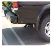
"MAKE SURE YOU HAVE A MINIMUM OF A 1  $\frac{1}{2}$ " CLEARANCE FROM ALL BRAKE LINES, TIRES, SHOCKS, FUEL LINES ETC."
