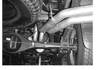
INSTALL THE DRIVERSIDE OVER AXLE TAILPIPE #D FROM THE REAR OF THE AXLE SLIP THE WELDED HANGERS INTO THE FACTORY RUBBER GROMMETS. THEN SLIP THE PIPE OVER THE OUTLET OF THE MUFFLER  $1\frac{1}{2}$  TO 2". USE CLAMP # G TO SERCURE TAILPIPES TO THE MUFFLER. DO NOT TIGHTEN.
