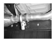
REMOVE STOCK EXHAUST BY UN-CLAMPING THE STOCK CLAMP AT THE HEADPIPE. BE CAREFUL NOT TO DAMAGE THIS CLAMP BECAUSE YOU NEED TO RE-USE IT. ONCE IT IS UN-CLAMPED, YOU WILL BE ABLE TO PULL THE STOCK EXHAUST OFF THE VEHICLE. MAKE SURE ALL FACTORY RUBBER GROMMETS ARE STILL IN FACTORY LOCATION, USE WD-40 TO AID YOU IN REMOVAL OF THE HANGERS FORM THE GROMMETS.
