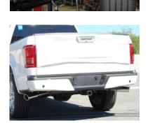
INSTALL YOUR STAINLESS TIPS AND CUT YOUR EXIT PIPES TO YOUR DESIRED LOOK AND LENGTH\*\* THEN GO BACK AND TIGHTEN ALL CLAMPS, ROTATE SYSTEM FOR BEST CLEARANCE BEFORE TIGHTENING.
