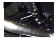
**6.** Install the driverside overaxle tailpipe #D into the muffler  $1\frac{1}{2}$ -2". Use clamp #H to secure. DO NOT TIGHTEN. Rotate until it meets with the rubber grommet. DO NOT TIGHTEN.
