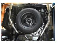
**7.** Next install the exit pipes #E. Use clamp #H to secure. DO NOT TIGHTEN. Rotate pipes to your desired look.
