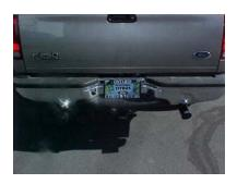
FINALLY AFTER TIGHTENING ALL CLAMPS FROM FRONT TO BACK AND MAKING SURE OF ALL CLEARENCES, INSTALL YOUR STAINLESS TIPS TO YOUR DESIRED LOOK.
