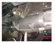
INSTALL MUFFLER #B ONTO HEADPIPE  $1\frac{1}{2}"$  TO 2". MUFFLER OUTLETS SHOULD BE ON TOP. ROTATE UNTIL LEVEL. SUPPORT MUFFLER WITH A JACK STAND. NEXT INSTALL FRONT MUFFLER HANGER #F INTO RUBBER GROMMETS, LOCATED NEXT TO MUFFLER INLET. THIS CLAMP WILL ALSO BE USED TO SECURE MUFFLER TO HEADPIPE. DO NOT TIGHTEN.
