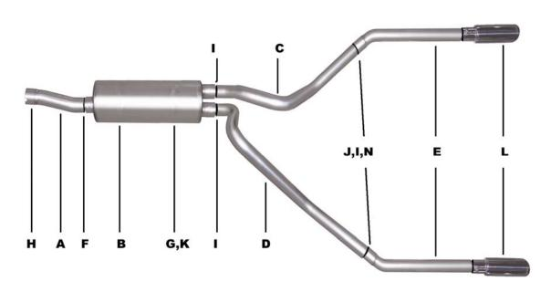
DO NOT REMOVE FACTORY EXTENSION PIPE BETWEEN MUFFLER AND CONVERTER
