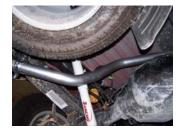
**7.** Install the driverside overaxle tailpipe #D into the muffler 1½-2". Use clamp #H to secure. DO NOT TIGHTEN. Rotate until it meets with metal hanger, use clamp #H to hold pipe. DO NOT TIGHTEN.
