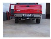
**9.** Install stainless steel tips. Clamp down. When you have everything in place, firmly tighten all bolts and clamps down securely. Use stainless steel cleaner and a Scotch Brite pad weekly to prevent tip from discoloration. Inspect all fasteners after 25-50 miles of operation and re-tighten as
