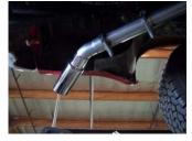
**8.** Next install the exit pipes #E. Use clamp #H, rotate pipes to the side. Trim ends of exitpipe to best fit your vehicle.
