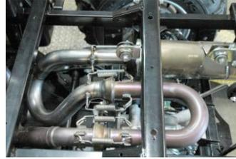
5. After muffer and mid-pipe are in place double check all springs and bolts are in place and tight.
