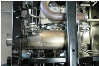
3. Now install Gibson muffler into stock location reusing factory bolts and using supplied 8mm nuts and lock washers. Tighten into place.
