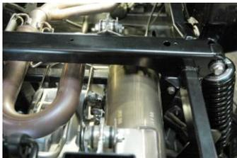
7. Remove 12 mm bolt to the left of the hanger bracket. Affix the new bracket with factory bolt. Rotate clockwise if pipe is sagging. Rotate counter clockwise if too high.
