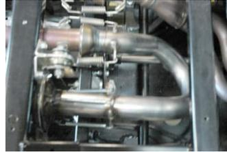
4. Next, install mid-pipe between factory headpipe and Gibson muffler. At factory connection reuse the 2 factory springs. At the Gibson inlet use the 3 supplied springs in addition to the donut gasket.
