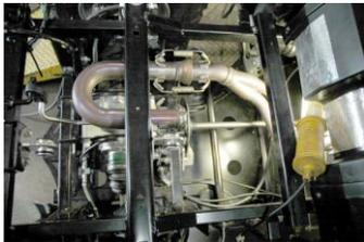
2. Now remove stock muffler using 12mm wrench or socket. Also disconnect the 2 factory exhaust springs.
