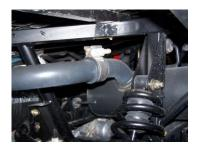
Remove the factory muffler by using the 15mm wrench or socket at the band clamp shown in the photo. Spraying a small amount of WD-40 will help with the removal of muffler from the rubber hangers
