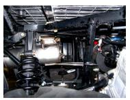
Item D. Slip the muffler in from the rear of the Rzr. Slip the lower long hangers into the rubber grommets first then pull back and slide the upper hanger into the single rubber grommet.
