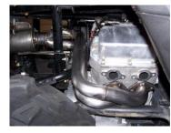
6. Slip item E dome gasket onto the outlet of the header collector and install the header assembly into the Rzr. Adjust the header tubes to allow the flanges to line up properly. Install supplied header bolts and factory gasket. Do not tighten.
