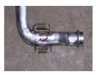
Use the factory springs to attach Item C to the header pipes. Item C the collector will have a top and a bottom. When looking at the collector from the side one way will have the single exit facing up wards at about a 10 degree angle or down ward. You want the single exit of the collector facing downward when slipping it onto the header pipes.
