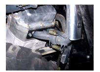
Next remove the entire exhaust. Do not damage the factory springs or Exhaust gaskets as they will be re used.
