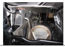
3. Next install the Gibson Muffler assembly. Install the top hanger mounts first then slide the inlet over the factory head pipe re using the factory gasket and springs. Once in position, install Headpipe and top muffler springs.
