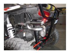
7. Once everything has been installed and tighten install your supplied Gibson tips. Slide the tips on to your desired look and tighten down. Check for 1" clearance around all pipes, rubber brake lines, shock boots, tires, etc... and go have fun!
