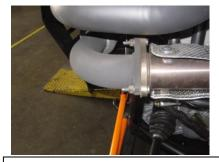
4. Next install the Gibson Muffler assembly. Install the top hanger mounts first then slide the inlet over the factory head pipe re using the factory gasket and nuts. Once in position, install head pipe and top muffler springs.
