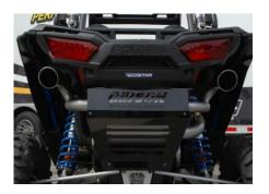
6. Install rear Gibson beauty plate. Use the factory bolts and supplied nylock nuts for the top two holes. Once they have been installed tighten the Gibson brackets at the Razor frame. Adjust plate for a level finish.
