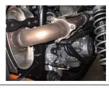
2. Once you have removed the heat shield remove the factory brackets and re install the Gibson supplied brackets #E using the factory bolts and factory location. Keep loose until final install.
