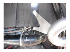
5. Bolt the tailpipe brackets to the rear under bed bracket. You will use Bolt Kit # B. Use the large fender washers on the back side of the top hole. You may have to loosen the factory bracket to adjust for fitment. Do not tighten until all bolts are installed. Install both sides.
