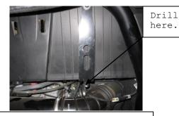
3. Next use a 1/4" drill bit to drill the hole for the tailpipe brackets. You will drill the lower threaded hole on the both driver and passenger side rear bed bracket. See above photo for location. Drill hole on both sides of the vehicle.
