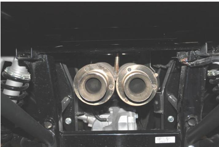
With the system securely in place in your desired position install the supplied clamp and tighten down the connection between the factory exhaust and the Gibson exhaust. It is important with this style clamp you place it to the edge of the Gibson pipe.
