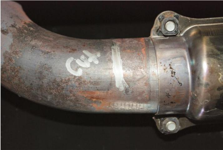
To begin the install of the Gibson Performance exhaust you will need to remove the factory rear portion of the skid plate. This will allow access to the factory head pipe where you will need to cut your header. You will measure 2" rear of the heat shield towards the back of the vehicle. This is the last heat shield before the exhaust makes the up turn towards the bottom of the vehicle.
