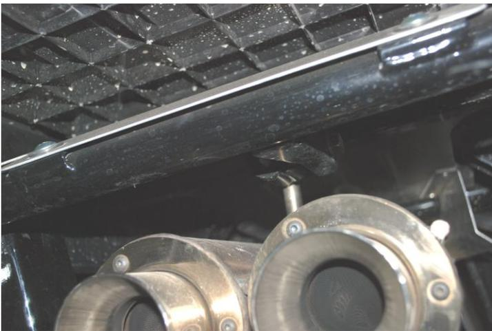
With your factory head pipe marked use a hack saw or saw zaw with safety glasses and make your cut. It is important that you have at least 2" of clamping surface for the Gibson Exhaust. Do your best to keep the cut as straight up and down as possible.
