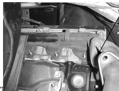
#6. FACTORY FLANGE CONNECTION. DISCONNECTING POINT.
