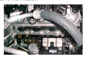
**9**) INSTALL THE NEW HEADER USING THE SUPPLIED HEAD GASKETS AND BOLTS. TIGHTEN THE GIBSON HEADERS FROM THE MIDDLE BOLTS TO THE OUTSIDE BOLTS.
