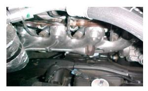
8) REMOVE THE SIX BOLTS ATTACHING THE MANIFOLD TO THE HEAD. REMOVE THE MANIFOLD.CLEAN THE SURFACE OF THE HEAD. REMOVE ANY CARBON DEPOSITS THAT MAY BE ON THE HEAD.PREPARE THE SUPPLIED HEADER BOLTS WITH ANTI-SEIZE TO THE THREADS. YOU WILL RE USE THE FACTORY DOME GASKET BETWEEN YOUR FACTORY MANIFOLD AND STOCK Y-PIPE
