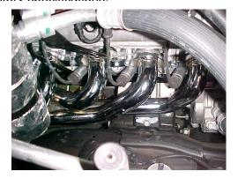
10) RE-INSTALL THE DIPSTICK TUBE. WRAP SPARK PLUG BOOT WITH HEAT WRAP PROVIDED AND RE-INSTALL. USING THE NUTS AND BOLTS PROVIDED, RECONNECT THE HEADERS TO THE STOCK EXHAUST UNDERNEATH THE VEHICLE.
