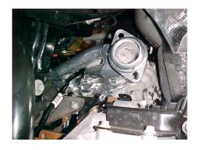
\*Note: Header Gasket has a top and bottom. The bottom is flat and should be aiming down.
