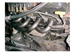
7. RE-INSTALL Y-PIPE WITH SUPPLIED HARDWARE AND TORQUE TO 30-35 FTS. CHECK ALL CONNECTIONS MAKING SURE THEY ARE ALL TIGHT. RE-INSTALL POSITIVE BATTERY CABLE.
