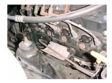
6. INSTALL SUPPLIED PASSENGER SIDE HEADER, GASKET AND SUPPLIED HARDWARE. TORQUE THE HEADER BOLTS TO 30-35 FTS. INSTALL THE ¼" BOLT, LOCK WASHER AND NUT ONTO THE BRACKET FOR THE DIP STICK. MOUNT THE DIP STICK TUBE TO HEADER USING THE BRACKET. INSTALL SUPPLIED HEAT WRAP ONTO SPARK PLUG WIRE #10 FOR HEAT PROTECTION.
