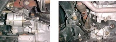
4. To remove the driver's side manifold. First remove the starter. Remove the driver's side manifold, studs and heat shields from the engine, through the top.
