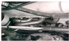
10.Reconnect the exhaust system to the header using the hardware provided.
