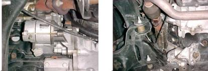
4. To remove the driver's side manifold. Fi arter. Remove the driver's side manifold, studs and heat shields from the engine, through the top.
