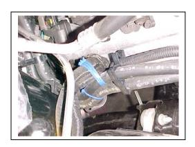
5. NOW INSTALL PASSENGER SIDE HEADER WITH SUPPLIED GASKET AND HARDWARE TORQUEING HEADER BOLTS TO 30 TO 35 FTLBS. NOW INSTALL Y-PIPE ASSEMBLY USING SUPPLIED HARDWARE. AFTER Y-PIPE IS INSTALLED DOUBLE CHECK ALL FASTNERS TO BE TIGHT. MAKE SURE YOU HAVE PROPER CLEARANCE FROM HOSES, WIRES; ALSO MAKING SURE HEAT WRAP IS SECURE!
