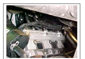
4. NOW NOTICE ON THE PASSENGER SIDE THAT YOUR TWO HEATER HOSES ARE CLOSE TO THE MANIFOLD. USE SUPPLIED Z-TIES TO TIE HEATER HOSES OUT OF THE WAY FROM THE LOG HEADER TO HELP PREVENT HEAT DAMAGE TO HOSES.
