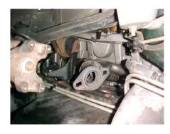
7. RE-INSTALL MOTOR MOUNT. **(ONLY ON CHEROKEE MODELS)** PLUG IN 02 SENSOR, INSTALL NEW SUPPLIED DONUT GASKET FOR HEADPIPE CONNECTION. THEN ATTACH HEADPIPE TO HEADER WITH NEW SUPPLIED EXHAUST DONUT. TORQUE HEADPIPE TO 30-35 FTS.
